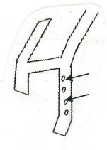
Caution: When hood is closed the snubber brackets on the hood must bottom out on cab bracket or the hood will not ride securely.
